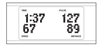
The lower left corner of the display will show your pedaling speed, in revolutions per minute.
